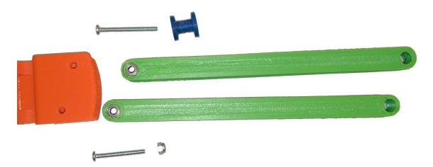
Note that in the hole nearest the edge, you will be using an M4x30 bolt that will terminate in a RubberBandPeg. In the other hole, you will be using an M4x25, and it will terminate in an M4 lock nut.
