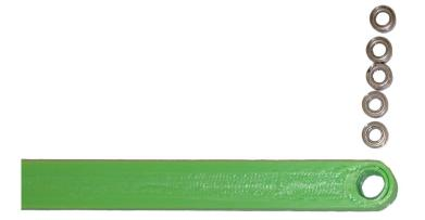
Once you have packed 5 bearings into each end of both rods, you will need to connect the Z-Rod to the LargeChainToZ\_Rod component.
