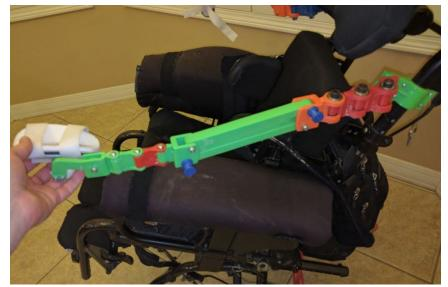
And now for the final part, attach the rubber bands to the pegs to add tension to the arm floats. You will have to tune the number of rubber bands for the individual who will be using the arm floats.
