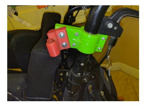
Here, you can see the MountAdapter attached to the PoleMount components. The PoleMount components are attached with 4 M4x15 bolts and lock nuts. The MountAdapter is attached using two M4x25 bolts, lock nuts. Two washers can also be used here to minimize the risk of splitting the MountAdapter.
